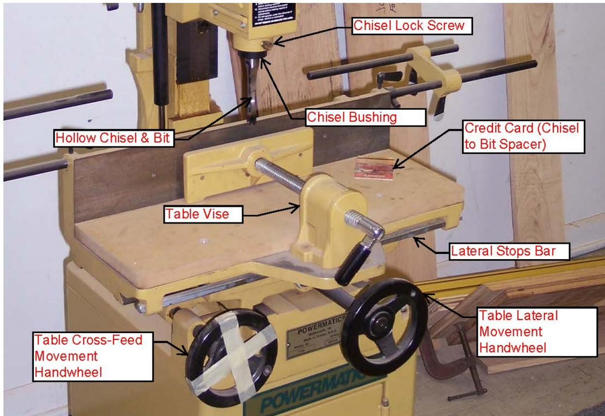
Install the bit and chisel. This procedure ensures that the drill bit has sufficient clearance from the chisel to prevent excessive heat and loss of temper due to friction between the bit and chisel.
