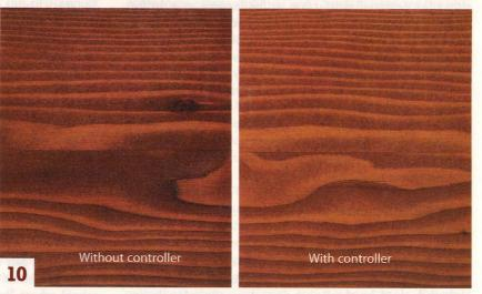
**Applied** in layers over stain controller, water-based dye and oil-based gel stain can be used to create a convincing old-wood "patina" on soft woods such as pine and fir, which are notoriously blotch-prone.
