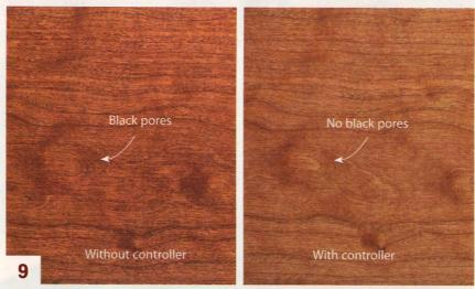
**Stain** controller helps to create a natural aged color on cherry by eliminating the tiny black pores that always appear when dark stain is applied on the raw wood.
