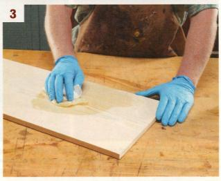
to provide a good balance. By my estimate, clear gel straight from the can that's allowed to dry overnight will produce approximately a 60% to 75% seal. Likewise, a 1:1 reduction will produce a 50% to 60% seal and a 2:1 reduction around 40% to 50%.
