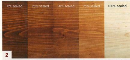
**Sealing** the wood to reduce blotching also reduces the stain's ability to add color. Using only the human eye as a meter, these estimates show a good balance at around 20% to 40% sealed.
