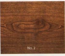
Results of the two methods for applying stain contoller described in Photos 3 and 4 and in the text are similarly effective but slightly different. The second method doesn't seal the wood guite as effectively, so the stain soaks in a little more.
