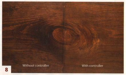
**Knots** add interesting figure rather than dark, unsightly blotching when a stain controller is applied before staining.
