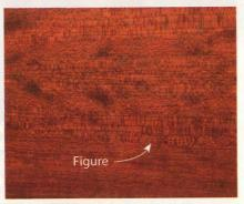
Water-based dye can cause blotching, just like any other coloring material. Thinned clear gel stain controller that has dried overnight minimizes unsightly blotching that obscures delicate figure.
