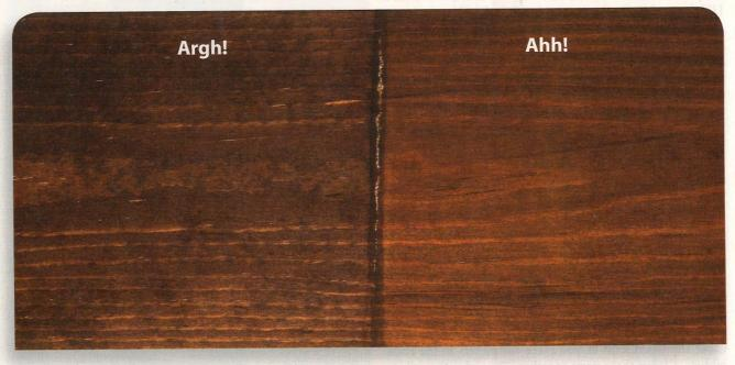
DISCOVERING UGLY BLOTCHING after applying stain is one of the worst finishing problems a woodworker can encounter-especially because the unsightly patches of dark, deeply absorbed color seem to appear out of nowhere, without warning. This problem can be very difficult, if not impossible to correct. Treating the wood with strong bleach usually doesn't work. Sanding until you remove all the unwanted dark patches is the only solution, and that can mean removing a lot of wood.
