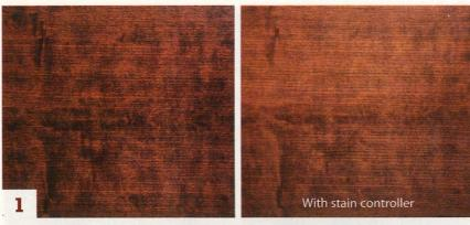
Stains that contain black pigment can cause blotching even when a stain controller is used to avoid it. Black pigment, used by some manufacturers as an inexpensive way to intensify color, can even be found in light-color stains.
