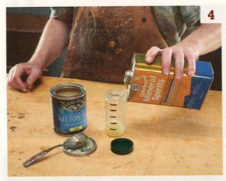
Make a universally compatible stain controller by thinning one part gel varnish with four parts mineral spirits. Apply the thinned controller generously, thoroughly rub off the excess and let the surface dry overnight before staining.
