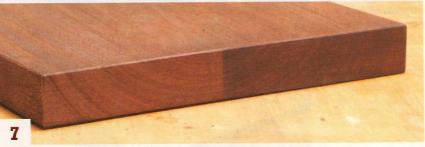
Match the color on the end of a stained workpiece with its surface by applying clear gel to the end grain only and then immediately applying any oil-based stain. This process also reveals the end grain's eye-catching figure.
