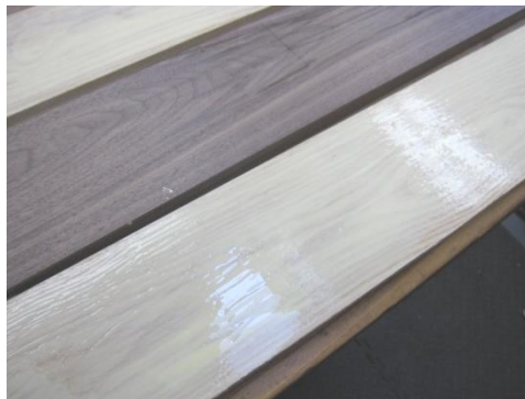
Glue Applied to Outer Boards
