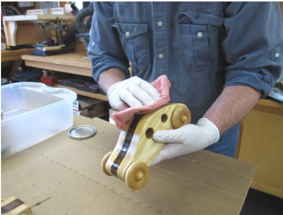
Wipe Off Excess Oil After Penetration
