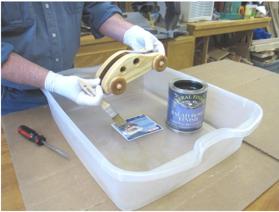
Make Sure Entire Vehicle is Wet with Oil Allow Oil to Penetrate for a Few Minutes
