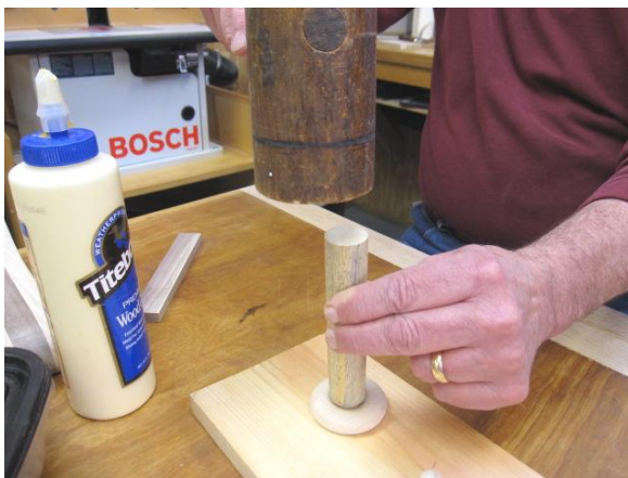
Use Sharp Blow to Seat Hubcap
