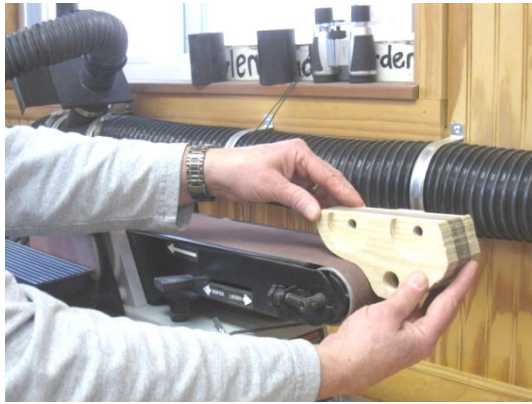
Use belt sander to shape & sand large contours, also flat edges and surfaces
