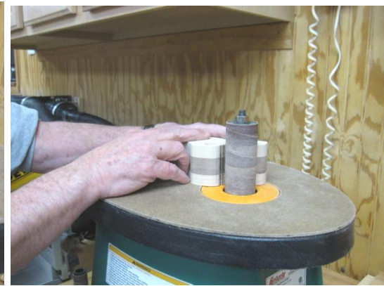
Use spindle sander to shape & sand smaller contours
