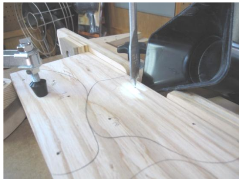
Drill Press Setup for Drilling Non-Recessed 7/16 in. dia. Axle Holes
