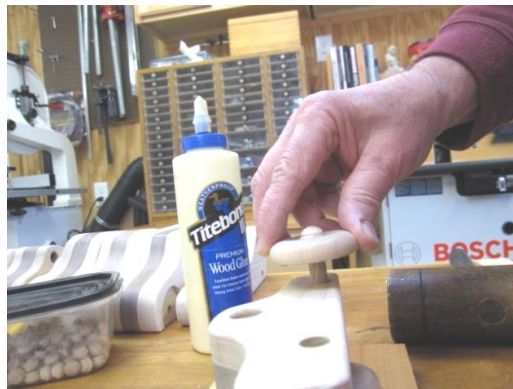
Place Top Wheel on Axle by Hand
