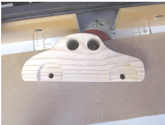
Rounding Over Window Openings
