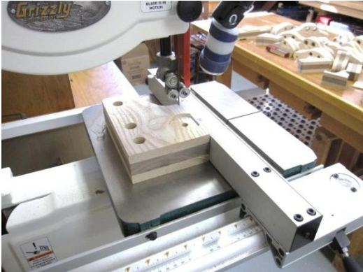
Use Fence to Cut Parallel Surfaces
