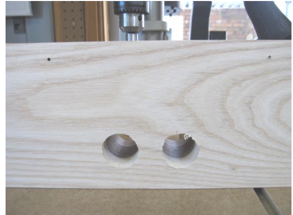
Backside Exit Holes (small holes at top)
