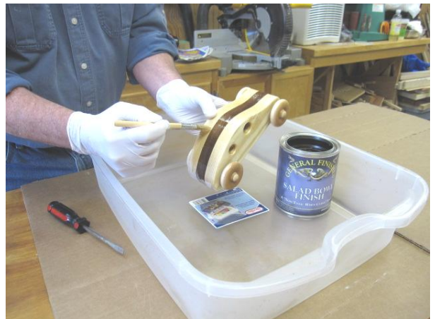
Flood all Surfaces, Check Wheels and Windows
