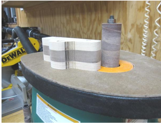
Use spindle sander to shape & sand smaller contours
