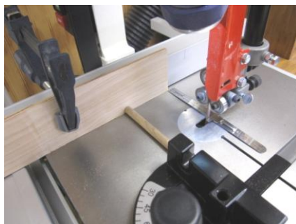
Band Saw Setup for Axle Cuts
