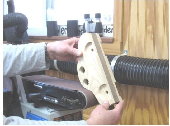
Use belt sander to shape & sand large contours, also flat edges and surfaces
