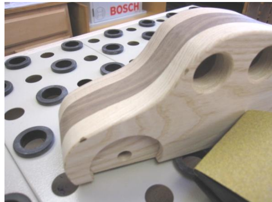
Remove Router Burn Marks
