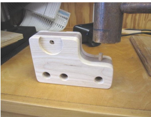
Cut Peg, Glue and Tap into Place on Trailer
