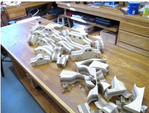
Batch Cutouts Completed (note scrap)
