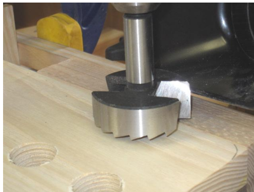
2 1/8 in. dia. Bit & Backer Board
