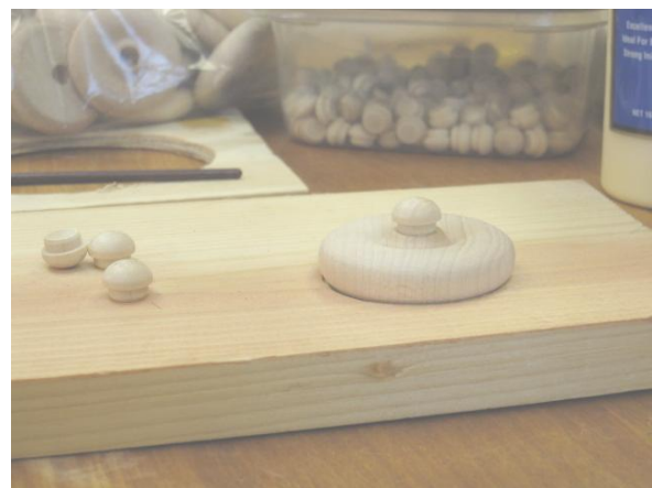
Center & Level Hubcap On Wheel
