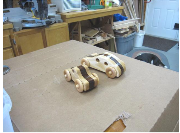
Make Sure Entire Vehicle is Wet with Oil Allow Oil to Penetrate for a Few Minutes
