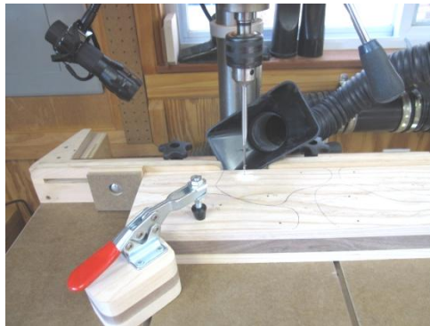
Drill Press Setup for Drilling Non-Recessed 7/16 in. dia. Axle Holes
