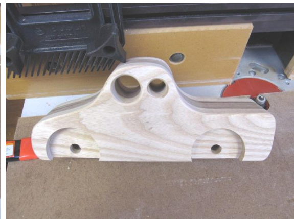
Rounding Edges Creates a Finished Look
