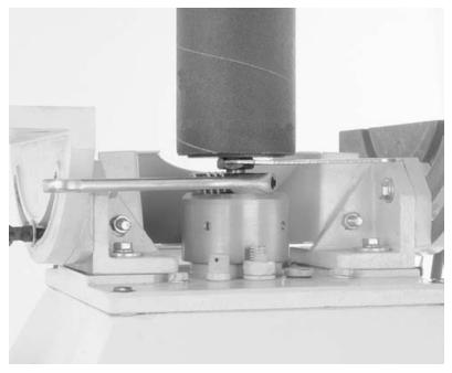
Drum removal - Table removed for clarity only
