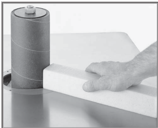
Figure 21. Routinely clean sanding sleeves with a rubber abrasive cleaning stick.
