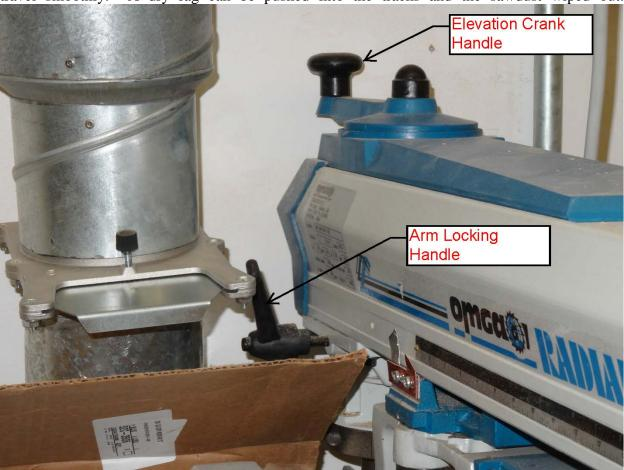
• Adjust the Miter angle of the saw (if any). (CAUTION! For all miter cuts, the standard aluminum fence (containing the scale and stops) must be replaced with a wood fence of the same size.
