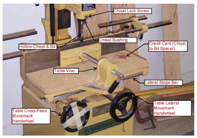
Install the bit and chisel. This procedure ensures that the drill bit has sufficient clearance from the chisel to prevent excessive heat and loss of temper due to friction between the bit and chisel.
