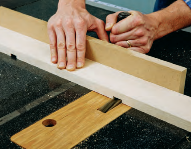
Plow a pair of 3/4"-wide dadoes across the filler strip to accommodate the table's leg pivot brackets. Set the width of these dadoes carefully so they provide a snug, friction fit for the brackets.
