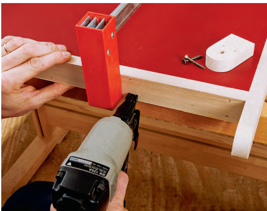
Wrap the table with hardwood edging, starting with the side pieces (pieces 7), then the front and finally the back. Secure with glue and pairs of 1 1/2" brad nails spaced approximately every 6". Complete the edging by gluing and screwing the table pivot brackets to the side edging.
