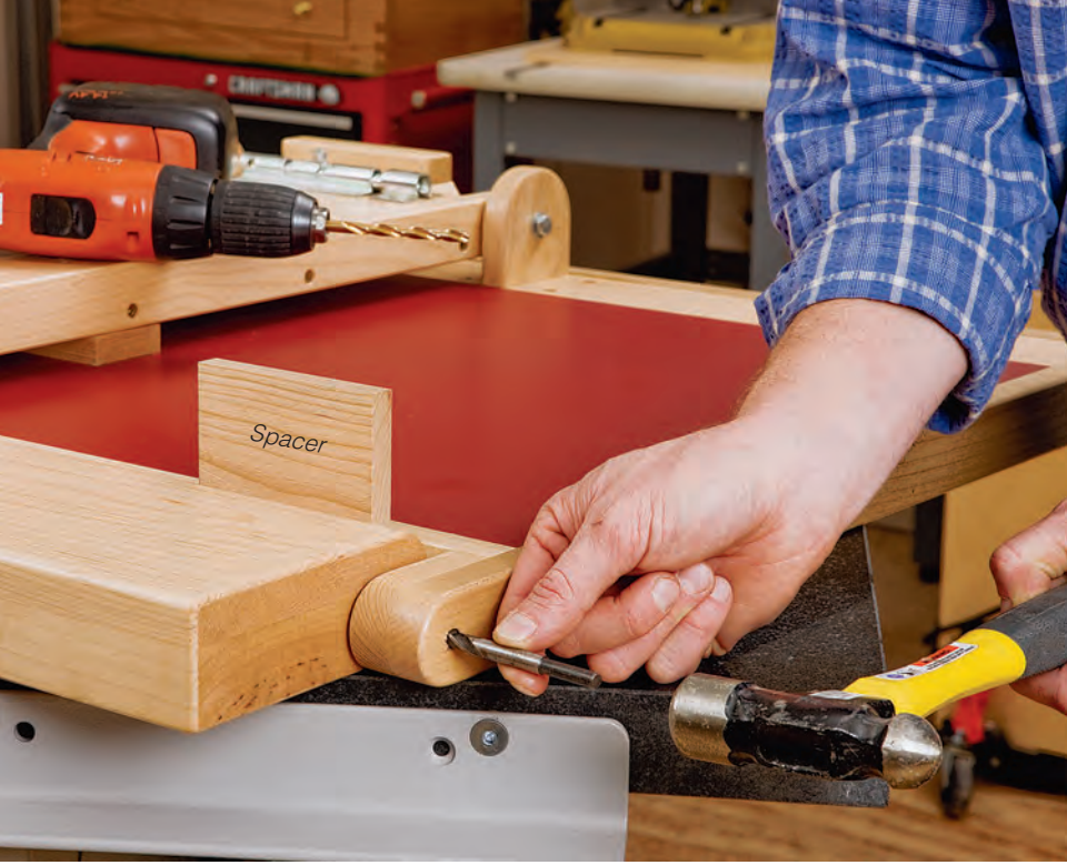
Mark centerpoints for long pivot screws on the ends of the mounting plate using a brad-point bit tapped through the table pivot holes. Hold the plate and table apart with a couple of 1/2" spacers.
