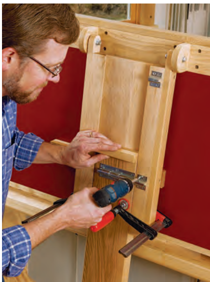
Screw the second metal receiver next to the first barrel bolt to set the open length of the leg. The top receiver keeps the leg retracted.
