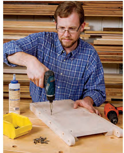
Fasten the pivoting leg braces to the leg's back panel, then glue and screw the beveled guide strips inside this leg housing.
