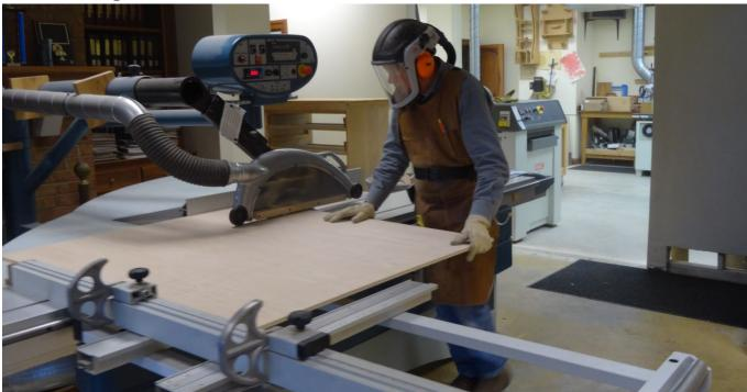
Cross-cut a piece of  $\frac{1}{2}$ " hardwood plywood 14-7/16" wide and the full 48" width of the plywood. Then cut to 8-1/16" long.
