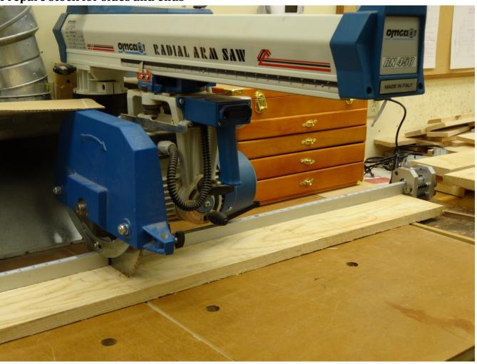
Cut the rough boards to 18" long. This is long enough to make one side or two ends. If the stock is clear and not twisted or bowed significantly, cut the stock to 36" long, which can yield two sides or four ends. Cut the stock to 27" and this will yield one side and one end. Keep in mind, the stock likely contains cracks and knots, so your yield may be less than expected.
