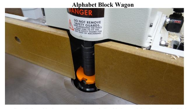
Install a raised panel back-cutter on the shaper spindle with the coved side down. Set the height of the cutter so that it cuts a 3/8" tenon that slips into the grooves cut into the sides and ends. Adjust the fence to minimize the opening and so that the width of the flat portion of the tenon is 5/16".
