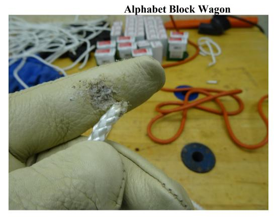
Then use your gloved fingers to bring the diameter of the end to a 1/4" tapered end. This must be done while the rope is hot.
