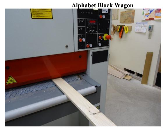
Sand both faces of the boards with 120 grit to a total thickness of  $0.625 \pm 0.010$ " (5/8").
