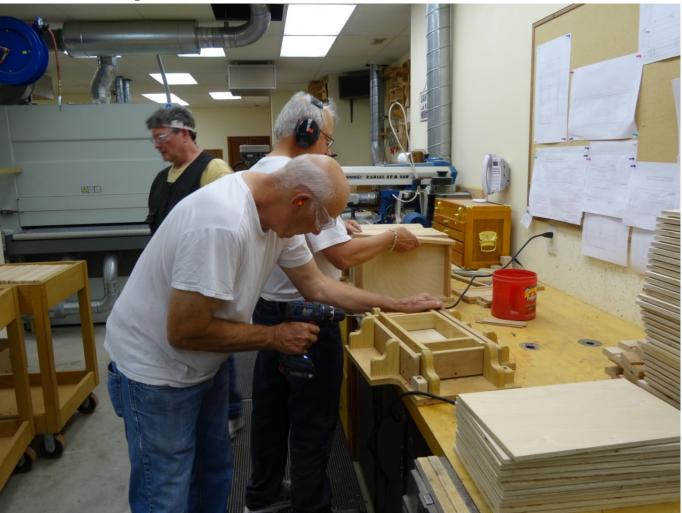
Assemble two sides, a bottom and two ends (with a rope hole in only one end). Then place the wagon in the assembly jig. Position the sides up against the side stops. Insert the frame that holds the sides and ends against the jig. Drill 7/64" pilot holes for the screws carefully aligned left and right to the center of the end. Install  $\#8 \times 1-1/2$ " flat head screws.
