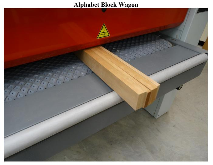
Sand both edges of each board to remove machine marks. Sand to a final height of 3.125" (3-1/8") for the sides and 2.875" (2-7/8") for the ends.
