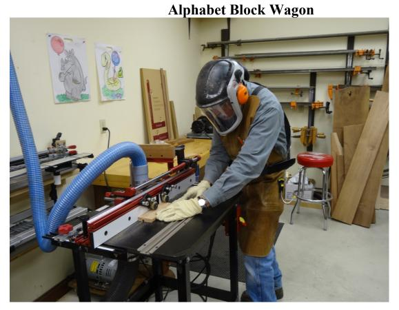
Select the best side of the end and face it up. Select the best edge and face it away from the fence. Cut a groove in each end piece. Feed the board slowly and use hold-down and feather boards to keep the end tight against the fence and table top.
