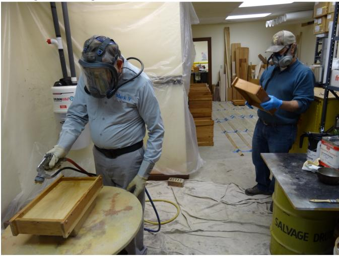
Suspend the wagon above the round-table using a cardboard box. Apply one coat of ML Campbell Krystal Semi-gloss post catalyzed varnish to the bottom and then the top sides of the box. Allow about 30 minutes and then sand the finish until it is smooth using a 3M Fine sanding pad. Use a brush head on the vacuum to remove the sanding dust. Then use a tack cloth for final cleaning. Apply a second coat of finish to the wagon box.
