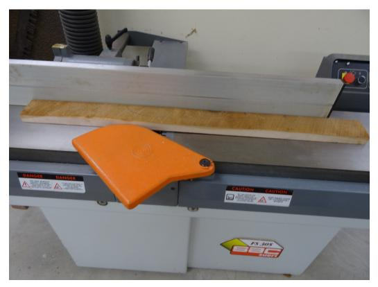
Re-joint the previously joined edge with the surfaced face of the board tight against the fence to ensure that it is square with the face.
