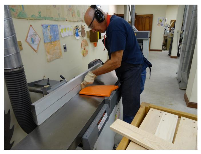
Joint the sawn edge of each board 1/32" to remove any saw marks.
