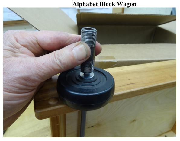
Use a ½" pipe nipple to hold the hubcap straight while tapping it in place.
