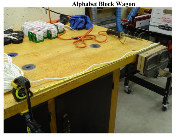
Cut 1/4" diamond braided polypropylene rope to 16" long using a soldering iron. Use the soldering iron to smooth the end of the rope.
