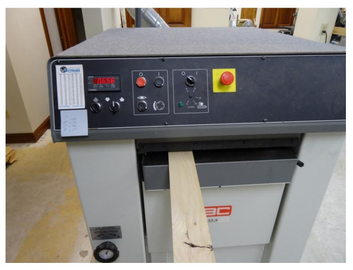
Plane the face of each board that was not jointed to approximately 0.650" thickness.
