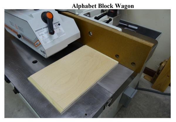
Using the power feeder, cut the tenons on both ends
