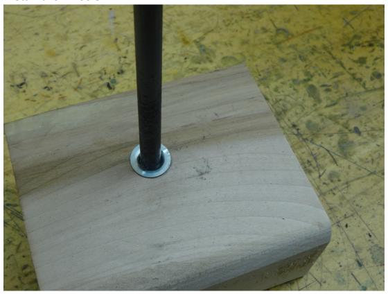
Place a hubcap in the hubcap jig and tap in a 5/16" cold rolled steel axle 12-13/16" long. Place a 5/16" SAE washer and then a 3" diameter, 1" wide soft rubber wheel followed by a second 5/16" SAE washer.
