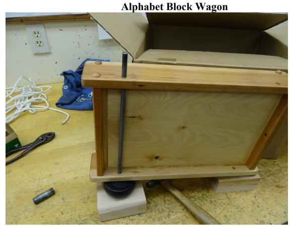
Slide the axle assembly into the wagon axle holes while maintaining the hubcap in the hubcap jig. Place a 5/16" SAE washer, wheel and second washer on the axle.
