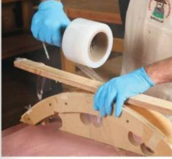
Into the vacuum. Use shrink wrap to keep the laminations together and positioned on the form. Once it's in the vacuum bag, the suction will pull the laminates tight to the form.
