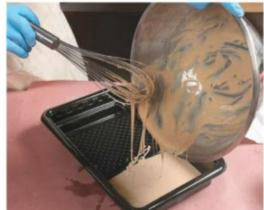
Unibond, a urea formaldehyde glue. is available in a twopart system, like epoxy. Once you've measured out the powder and the liquid (1 part powder to 4 parts liquid or 1:6 for a slower dry time) mix them together. Van Dyke pours the mixture into a paint tray and rolls it onto the work. Unibond cures to a rigid, strong bond, making it a solid choice for bent laminations. Roll the glue on one side of each lamination as you stack them.
