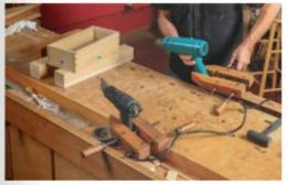
Disassemble a dried joint. With liquid hide glue, it's easy to take a joint apart after the glue sets. In this case, the dovetailed box was glued up before it had a groove to hold the bottom. No problem. Just heat the corners until the glue softens and the joints come apart. Van Dyke uses opposing wedges to force the box open. He sets a pair of wedges on either side, and uses clamp pressure to move them toward each other, pushing the joint apart.
