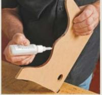
Seal and harden. Spreading medium thick CA glue and spraying an accelerator on MDF templates seals the edges and hardens them, allowing a single template to last through years of repeated use.
