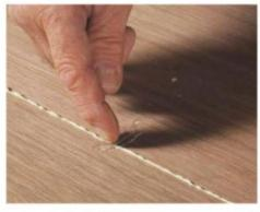
A level glue-up makes flattening easier later. Use spring clamps to hold the boards flush, testing flatness with a finger. Before adding clamps across the top, scrape off any squeezeout. This allows the glue joint to dry faster. Add the top clamps, then flip the panel and remove the glue from the bottom as well.
