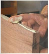
Don't waste any time. Because yellow glue skins over quickly, Van Dyke starts by running a bead of glue along both edges to be joined. It is then quickly spread with a finger. Rubbing both edges back and forth ensures a thin, even layer on both surfaces.
