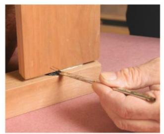
A smart glue-up strategy. Brush the glue into the mortise, and around the tenon, putting a thin coat on the end grain shoulders of the tenons. Before you seat the tenon all the way in the mortise, stop and brush out the roll of glue that forms as the tenon goes into the mortise. This will help eliminate
