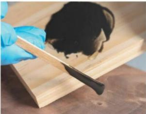
Mimic a natural defect. Rather than trying to hide a void by camouflaging it, you can use tinted epoxy to fill a hole and imitate naturally occurring flaws like knots or pitch. Mix equal parts of 5-minute epoxy and add a dab of oil pigment to tint. Drop the colored epoxy mixture into the defect, and let it cure, then scrape it flush. Let it fully cure overnight before scraping and finishing.
