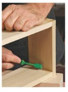
Cleanup is easy. Water is all it takes. Whether you are cleaning squeeze-out while it's still wet or after it has been dry for days, the answer is always the same. Use warm water on a rag or brush and you can work the glue away.
