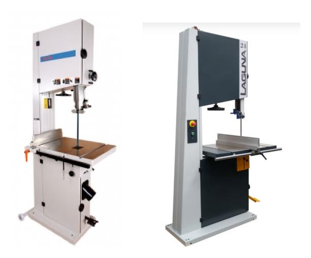
The Band Saw has a thin vertical blade that allows cutting curves, resawing, and large depth cuts on thick material. To avoid accidents, the following operational safety rules must be observed by everyone using the CLUB 20" Mini Max Band Saw. Failure to follow the safety rules will result in a loss of shop privileges.
