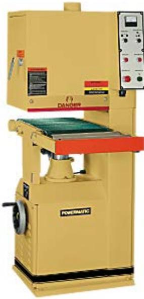
The wide belt sander is used to quickly sand the surfaces of boards to a very smooth finish. It uses a sanding belt that is 17” wide to sand boards up to 16” wide in a single pass. Boards up to 32” wide can be sanded in two passes. To avoid accidents, the following operational safety rules must be observed by everyone using the Powermatic wide belt sander. Failure to follow the safety rules will result in a loss of shop privileges.
