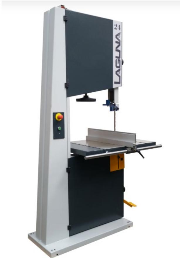
The Band Saw has a thin vertical blade that allows cutting curves, resawing, and large depth cuts on thick material. To avoid accidents, the following operational safety rules must be observed by everyone using the CLUB 20” Mini Max Band Saw. Failure to follow the safety rules will result in a loss of shop privileges.
